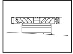
6. Check level of reducer in both directions. Make any necessary adjustments required using 1/8" shim plate (see #4).
