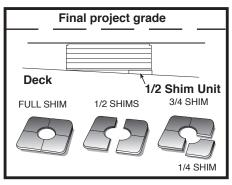
Use 1/8" shim plate under reducer, when required, to level with laser line. (Shims are scored to allow field cutting)
