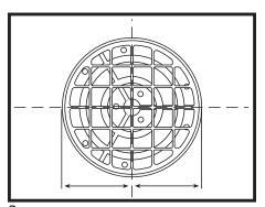
3. Center reducer unit on chalk line(s) previously established for paver layout.
