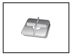
9. When height clearance is limited, the use of 1/8" shim plates with 3/16" or 1/8" spacers may be required.
