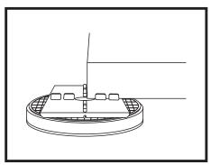
7. Place Terra-Tab paver support unit on top of reducer and install pavers. See back of instructions for details.
