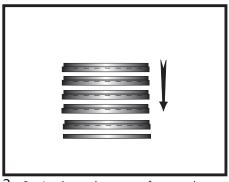
Setting base plate on surface, stack reducer rings over each other until required height is approximately reached.
