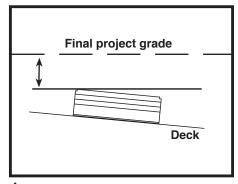
Use laser line or equivalent to establish final project grade. Subtract thickness of paver and suppot unit (Terra-Tab) to determine final reducer height required.
